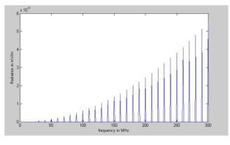
Figure 04: Radiation of Electric field intensity due to dipole (10mA)
