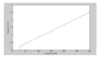
Figure 06 Radiation of Electric field intensity due to dipole(20mA)
