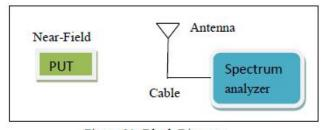
Figure 01: Block Diagram.
