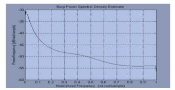
Figure 12: PSD of Electric field
