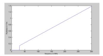
Figure 08: Radiation of Electric field intensity due to dipole(10mA)
